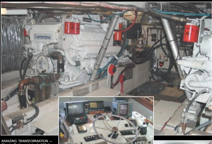
Check Out's original 420 hp Cummins BT 903 diesels (top) were more than 20 years old. The new electronically controlled engines that replaced them — 635 hp Cummins QSM 11 diesels — offer bet-
